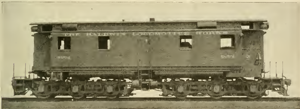
Diesel Oil-Electric Locomotive Built by Baldwin Locomotive Works Equipped With Westinghouse Apparatus
